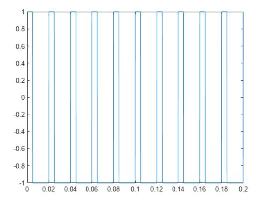
Use the dutycycle function to verify that the duty cycle of the square wave is the specified value. Use the function with no output arguments to plot the waveform, the location of the mid-reference level instants, the associated reference levels, the state levels, and the associated lower and upper state boundaries.
